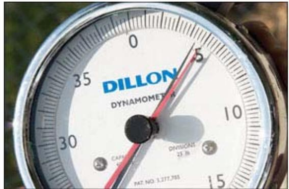
In determining proper scope, testers took water depth and the height of the winch above the water's surface into account. A crew aboard a *PS* test boat carefully dropped the anchor and then retrieved it after each load test was done. Anchors often came up with heavy mud clinging to them, so testers made sure each anchor was clean before the next test.
