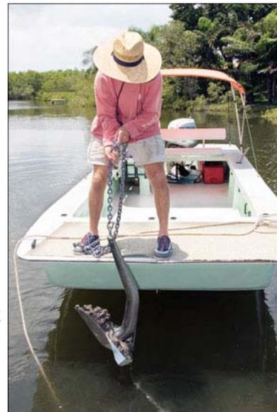
At 48 pounds, the Quickline anchor would normally be wrestled up with a windlass. Weighted with lead so that it lands ready to set, the anchor quickly pushed the needle on the Dillon dynamometer to the 500-pound mark.
